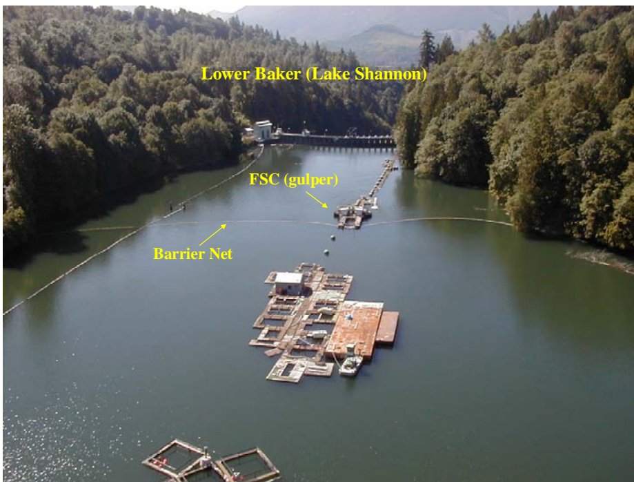
Figure 3. Lower Baker forebay aerial showing existing surface collector, net, trap, and defunct pens.
